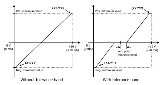
The default *Minimum Frequency* **418** or *Minimum Reference Percentage* **518** extends the parameterized tolerance band to the hysteresis.
