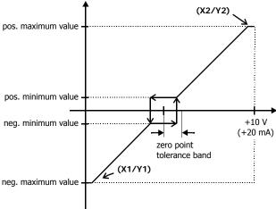
Tolerance band with set maximum frequency
