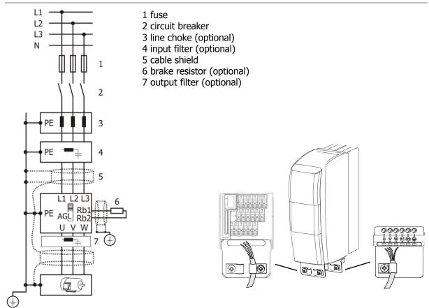
Optional shield sheets can be used for the cable shielding. Refer to chapter 12.2 "Shield sheets".
