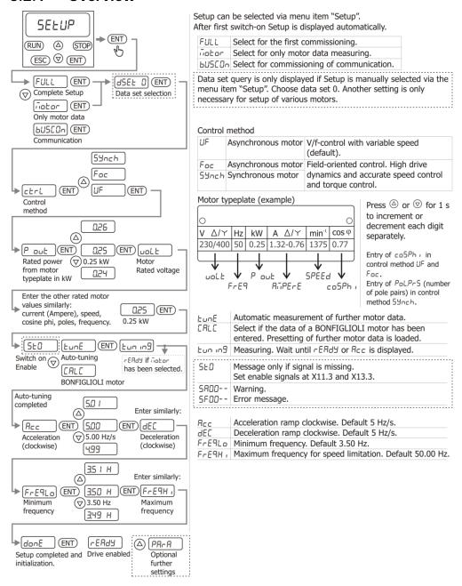
**Note**: The overview shows the sequence for an asynchronous motor. When commissioning synchronous servo motors, the motor type (BCR, BTD, "Other") has to be selected additionally and the order of the entry of the motor parameters is adjusted.
