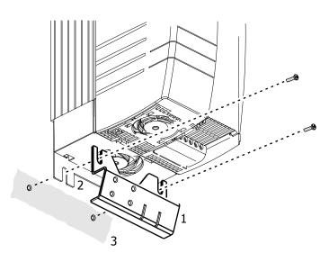
Assemble the shield sheet (1) together with the fixing bracket (2) onto the mounting plate (3).
