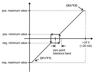
Tolerance band with set maximum frequency
