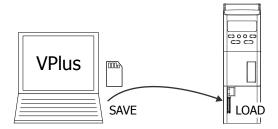
Activate in the Saving mask for the usage on a MMC card always the function "Save to Multimedia Card". To save a file for a MMC card only file names in the range from 0001 to 9999 are allowed to be used. The file names must be entered in the format "four-digit" + file extension for the usage on a MMC card.
