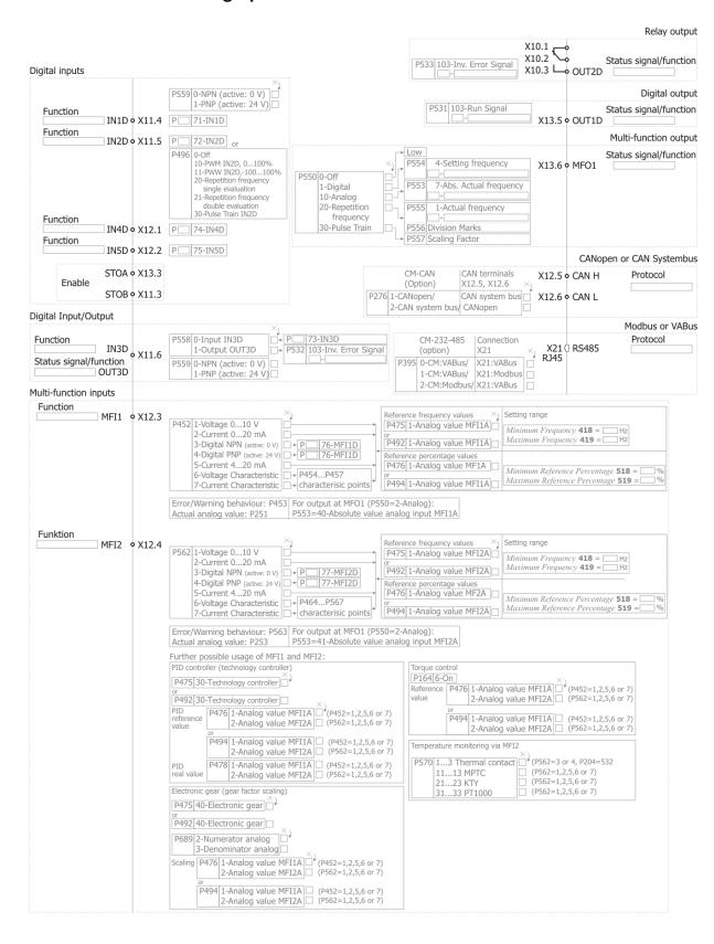
The block diagram only shows a selection of possible uses of the inputs and outputs.
