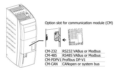
Further communications modules are listed in chapter 3.1 "Inverter type and warning signs on the device". The VABus protocol is used for communication with the PC software VPlus for parameter settings, monitoring and diagnosis.
