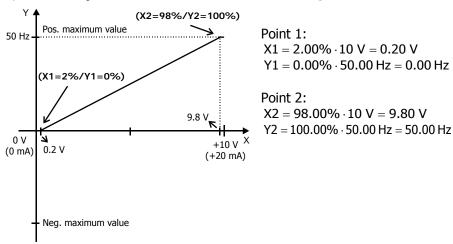
The characteristic can be adjusted via parameters 454 ... 457 of the application.
