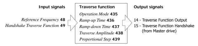
Signal "14 - Traverse Function Output" is added to the reference frequency value. During traverse operation, the configured traverse parameter values cannot be changed. The source of the handshake signal is selected via *Handshake Traverse Function* **49**.
