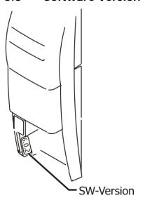
The Software version plate is situated right from the memory card slot and left from the Control terminals.
