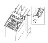
For connection to IT mains, pull out the plug-type jumper.
