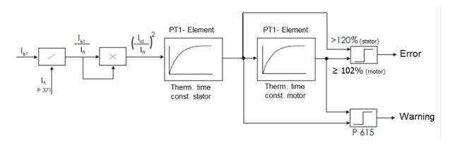
The output of the first PT1 element is linked to the input of the second PT1 element which includes the thermal motor time constant. This output may be permanently 100%.
