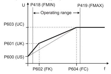
(FMIN): Minimum Frequency 418, (FMAX): Maximum Frequency 419,
