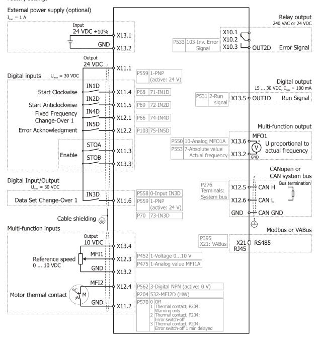
Comply with the technical data of control terminals: See chapter 11.3 "Control electronics".
