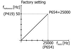
The Speed Control is always limited by the Minimum Frequency (P418) and Maximum Frequency (P419).
