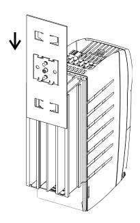
During the assembly a good contacting of the frequency inverter to the DIN rail must be assured. A good PE-connection of the frequency inverter to the assembly material and the DIN rail requires metallic conducting contact.
