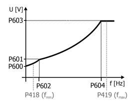
After switching over to the quadratic characteristic, the characteristic is defined by the following parameters:
