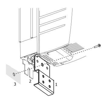
Assemble the shield sheet (1) together with the fixing bracket (2) onto the mounting plate (3).
