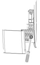
Loosen the lower screw slightly (don't turn out completely).
