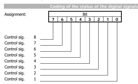
A decimal value is displayed, indicating the status of the digital signals in bits after conversion into a binary figure.
