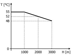
Reduction of cooling agent temperature T depending on installation altitude H.
